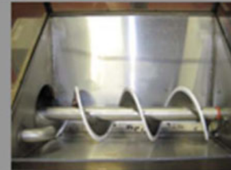
Photo Above: Shows need for additional machine guarding
